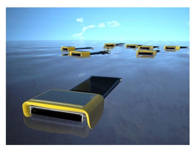
Seaswarm is pretty similar to Ocean Therapy Solutions' device which filters crude oil from sea water, because it is designed to specifically siphon crude oil from sea water at a spill site. Ocean Therapy Solutions' largest device could siphon up to 200 gallons a minute, but Seaswarm claim that as a collective group, their machines can work together to clean even larger areas of ocean.  $(\pi \epsilon \rho \iota \sigma \sigma \delta \tau \epsilon \rho \alpha ...)$
